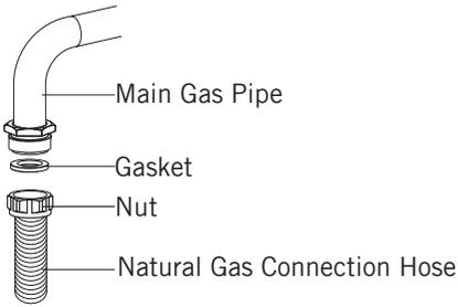
**2.** Natural gas connection should be done by authorized service. For natural gas connection, place gasket in the nut at the edge of natural gas connection hose. To install the hose on main gas pipe, turn the nut. Complete the connection by making gas leakage control.
