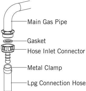
1. For LPG (cylinder) connection, affix metal clamp on the hose coming from LPG cylinder. Affix an edge of the hose on hose inlet connector behind the appliance by pushing to end through heating the hose in boiled water. Afterward, bring the clamp towards end section of the hose and tighten it with screwdriver. The gasket and hose inlet connector required for connection is as the picture shown below.
